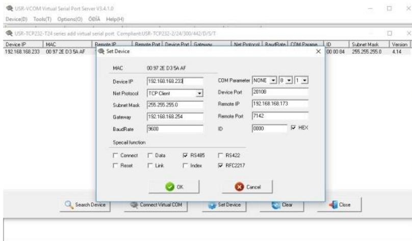
**Device IP** -> Ethernet device IP address (assign a free network address)
